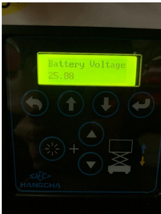
Battery Voltage / 电池电压
